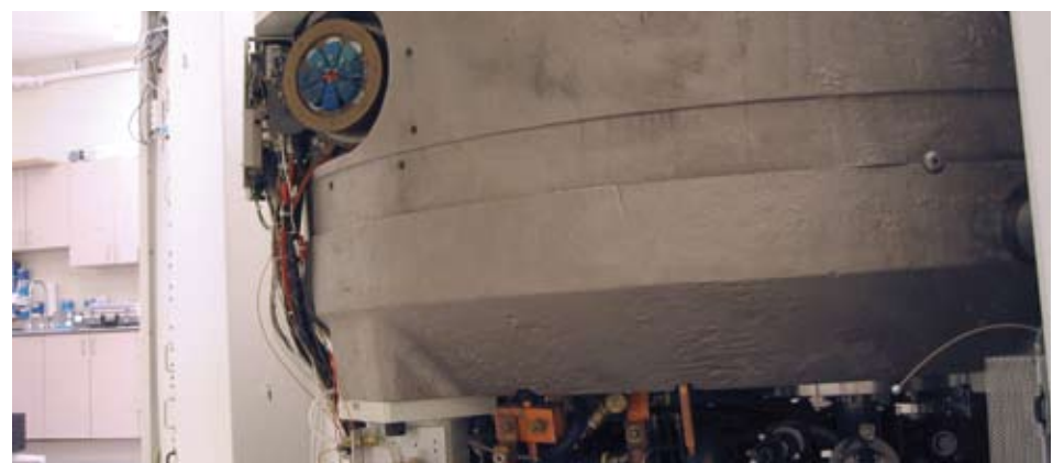
Where tracers come from: The Heart Institute's cyclotron produces short-lived radioactive isotopes by aiming a stream of accelerated protons at a target substance. The target is the ring on the left with the blue flower-like pattern. A second target will be installed in the coming months to double the cyclotron's production capacity.
