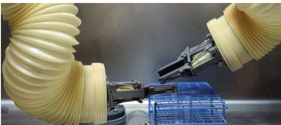
Inside the hot cell, remote arms allow scientists to manipulate heavy objects as well as fragile test tubes. It takes a good deal of practice and hand-eye co-ordination to prepare a sample from behind two inches of shielding.
