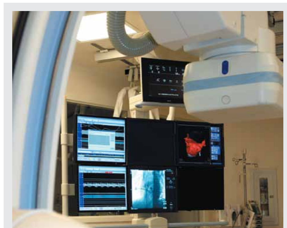
The new DynaCT system generates real-time 3-D images that help Heart Institute physicians diagnose and target treatment of dangerous arrhythmias. The technology makes it possible to conduct the diagnostic imaging and ablation treatment in a single procedure, reducing the need for multiple patient visits and likely reducing the overall radiation dose.
